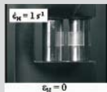
Visualization of an extensional experiment on a polyolefin melt
