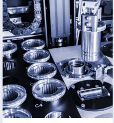
Pre-tempering unit for increased throughput An automated Peltier unit pre-tempers the sample before it's placed into the rheometer, shortening the tempering time in the rheometer and increasing throughput.
