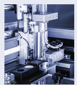
pH station for additional sample analysis pH measurements, pH probe cleaning, and reference measurements performance checks - it's all automated.
