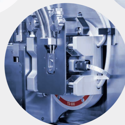
Stress/strain investigations with the Tensile Stage
