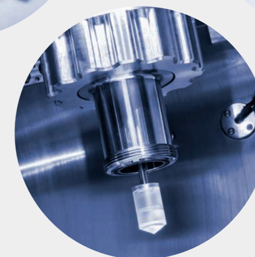
RheoSAXS module for combined rheology and scattering experiments on liquids
