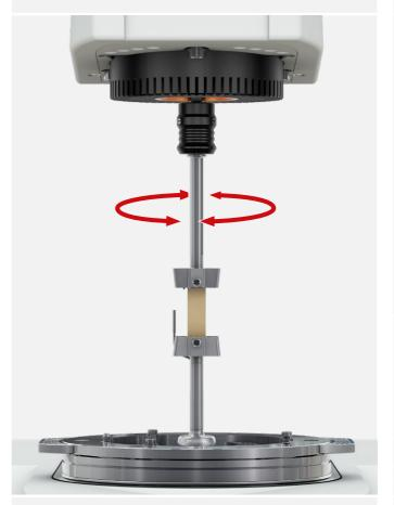
In this mode the linear drive is brought into a fixed position, while the rotational drive is used to control shear strain or shear stress. In combination with available fixtures such as solid circular and rectangular fixtures (SCF, SRF) and plate-plate or cone-plate geometries, this option opens up the possibility to perform dynamic mechanical analysis in torsion and also rheological measurements.
