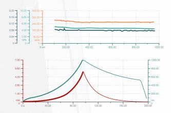
An example of sinus mode (dynamic mechanical analysis, DMA) performed by a nanoindentation tester.
