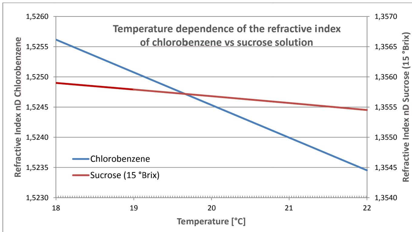
Figure 1: Influence of temperature on the refractive index of chloro-benzene and sucrose solution.
