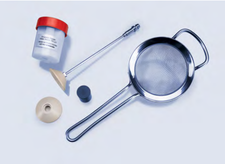
Simple and safe measurement method for characterizing the envelope density of solids with a sample size ranging from 0.3 cm³ to 25 cm³, by using a reusable, free-flowing displacement powder. Precise volume measurement with a repeatability of up to 1 % is ensured with a sample quantity of at least 25 % of the total filling volume. In combination with gas pycnometry measurements, the absolute density, porosity, and specific pore volume of solid materials can be determined.
