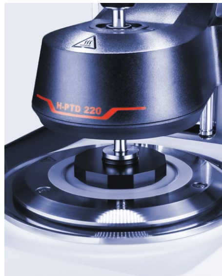
Peltier temperature control for parallel-plate systems (P-PTD 220) and hood for up to 220 °C (H-PTD 220)
