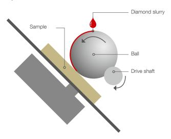
A small crater is ground into a coating with a ball of known geometry, providing a tapered cross-section of the film when viewed under an optical microscope. In this way Calotest instruments measure the thickness of coatings in a very short time of just 1 to 2 minutes.
