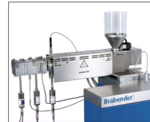
Measuring extruder / Extrusiograph 19/25, Application: Thermoplastics
