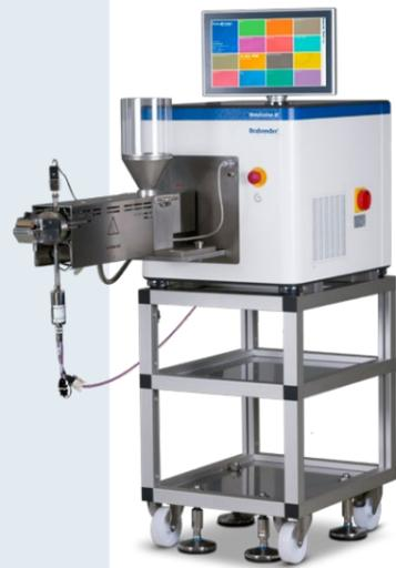
MetaStation 4E with measuring extruder 19/25 and ribbon die head
