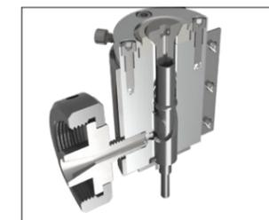
Film blowing die head with cooling ring
