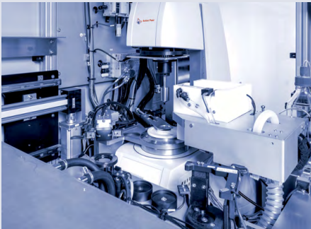
High-precision rheometer and cleaning unit for upper measurement geometry
