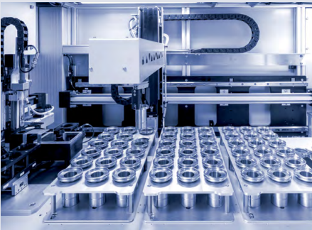
3-axis handling system with cup gripper / 54 CC27 cups
