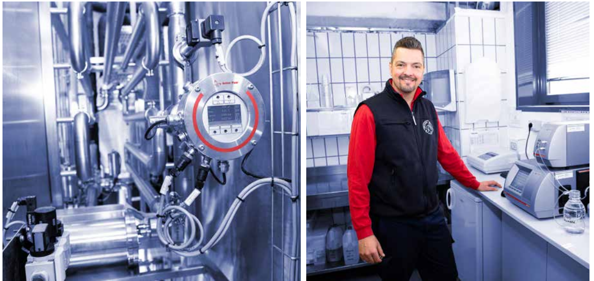
The Carbo 510 sensor monitoring CO 2 online and brewmaster Pausler with the DMA M-Alcolyzer setup in the lab
