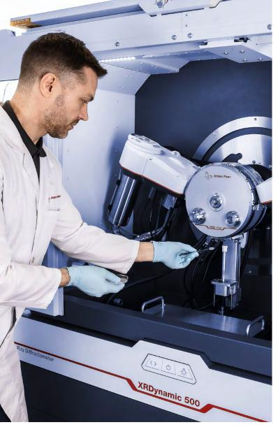
The HTK 1500 High-Temperature Chamber is the new benchmark of environmental heaters for X-ray diffraction (XRD). It allows you to homogeneously heat all types of sample materials, including crystalline powders and bulk samples, up to 1,500 °C. The position of the heating rods, together with a highly accurate temperature measurement, makes HTK 1500 the only 'true' environmental heater up to 1,500 °C.
