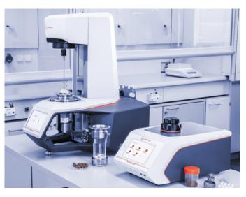
→ **Additional solution:** Determine the absolute density and porosity of the sample with Anton Paar's Ultrapyc gas pycnometer series.
