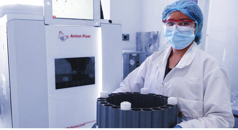
→ Multiwave 5000 eliminates operator exposure to toxic and hazardous vapors.
