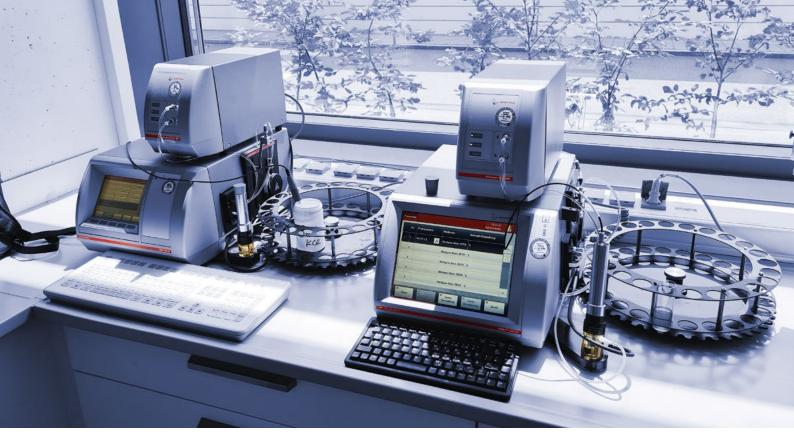
→ For many years, all beer samples at Hofbräu München have been measured by Anton Paar's Alcolyzer Beer Analyzing Systems, delivering all key parameters relevant for QC with one sample filling, at the push of a button.
