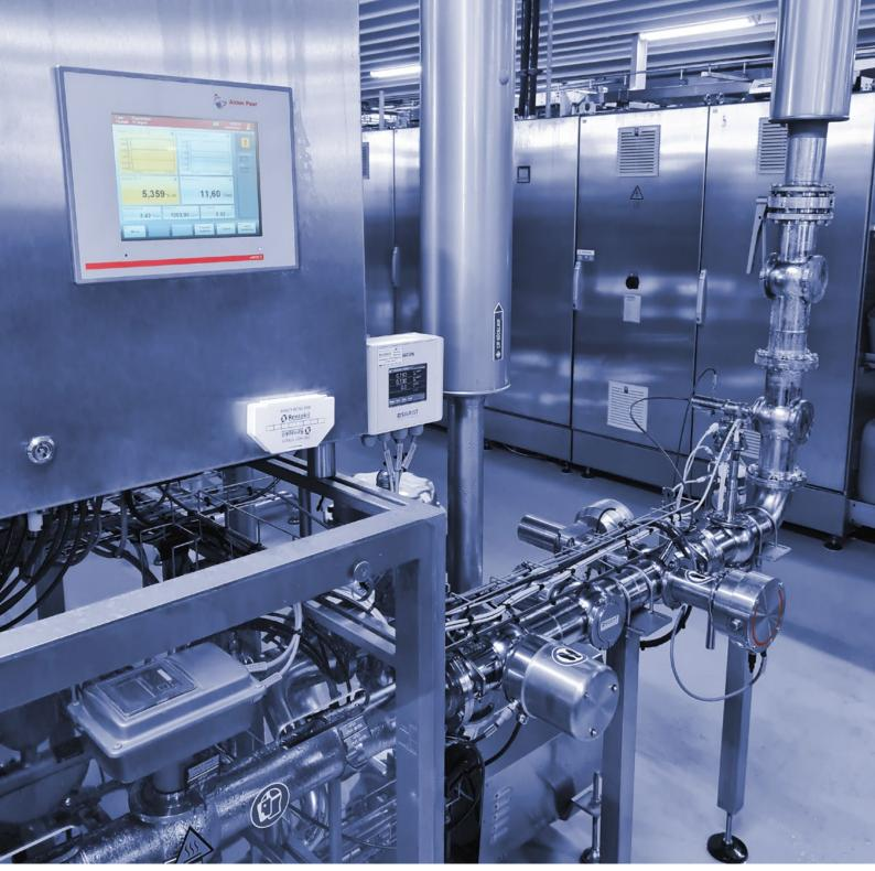
→ At Hofbräu München, inline sensors are calibrated and adjusted with values measured by lab instruments at the push of a button via Anton Paar's Davis 5 software.
