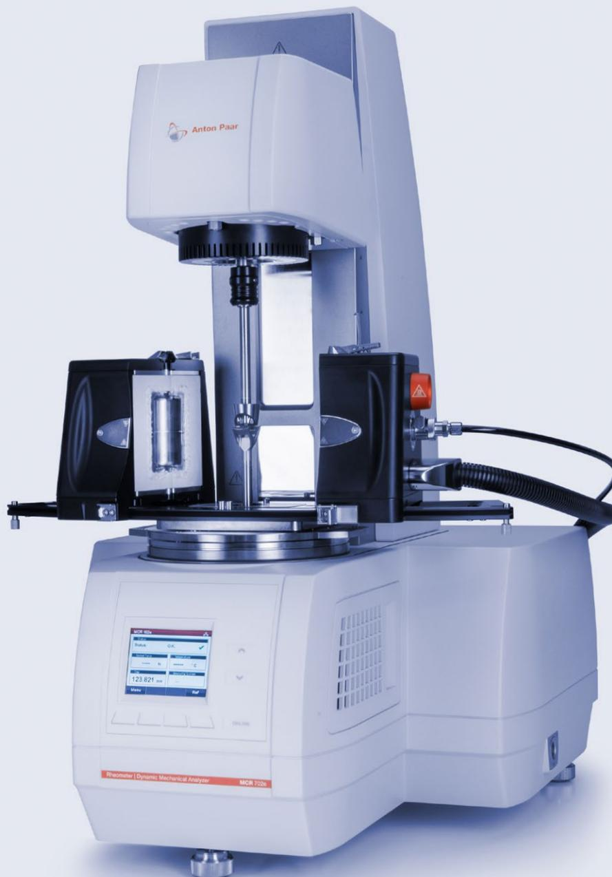
Anton Paar's high-temperature rheology portfolio enables you to run rheological tests, dynamic-mechanical analysis and liquid density measurements of samples up to 1,800 °C.
