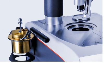
The PMA 500/300 series is a closed-cup flash point tester equipped with premium technology and a modern design. The top-performing instrument determines expected flash points from above ambient temperature up to 410 °C (PMA 500) and 370 °C (PMA 300), respectively. It guarantees straightforward, automated handling, maximum safety, and unrivaled usability in combination with a self-explanatory user interface.
