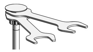
When mounting or dismounting the disposable plate **always remove** the shaft from the measuring system coupling. Excessive lateral forces might damage the measuring drive.
