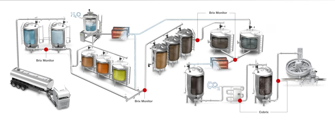
In-line beverage analyzers in the wine manufacturing process
