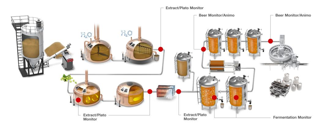
In-line beverage analyzers in the Hard Seltzer manufacturing process
