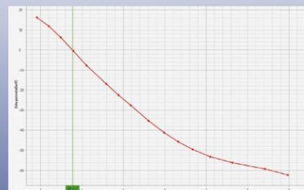
pH scan indicating the isoelectric point (pH vs. zeta potential)
