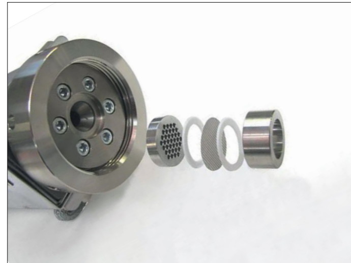
Structure of the pressure filter test consisting of perforated plate and filter sieves
