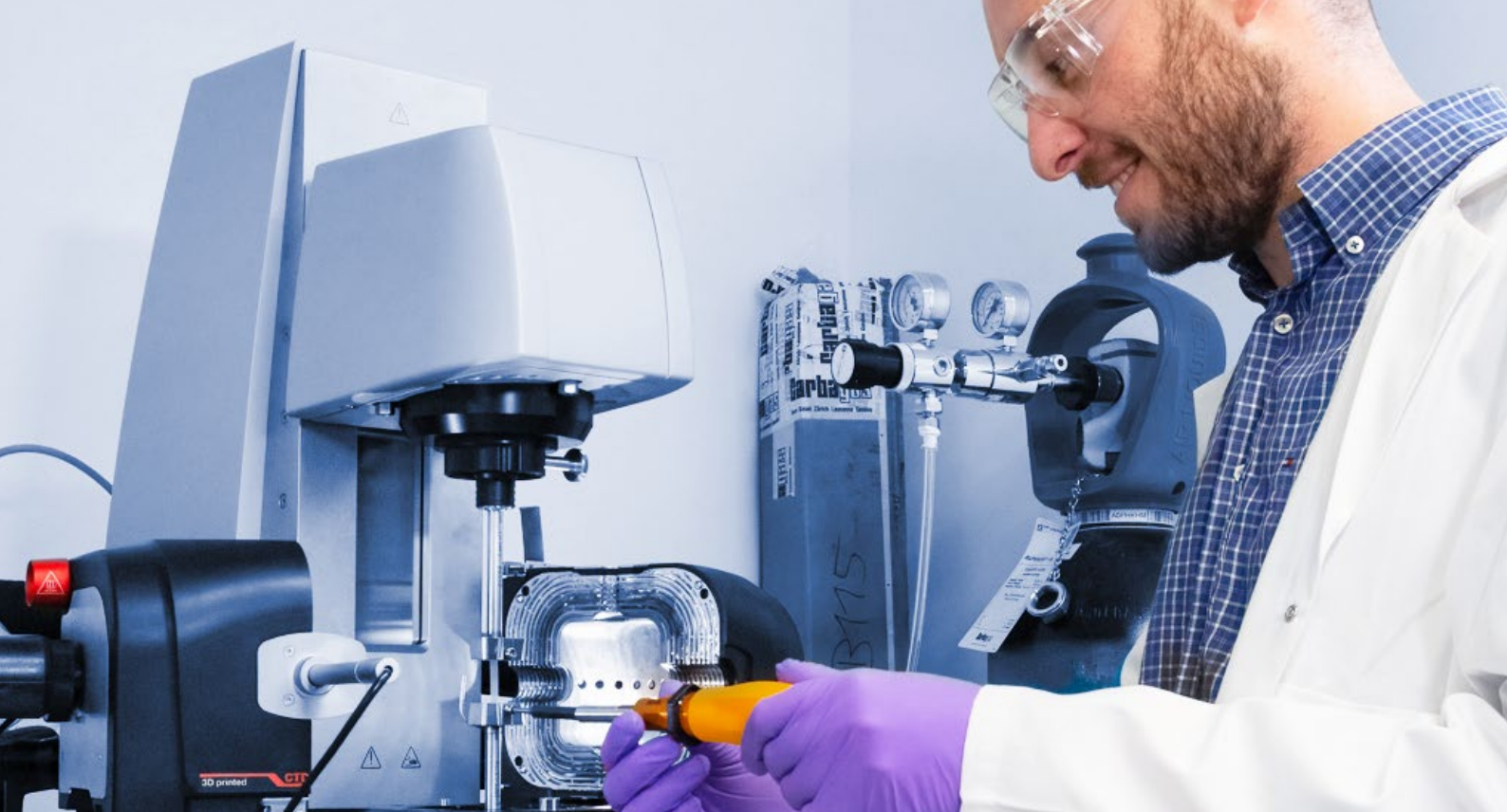
→ Solid Rectangular Fixture for DMA in tension and torsion
