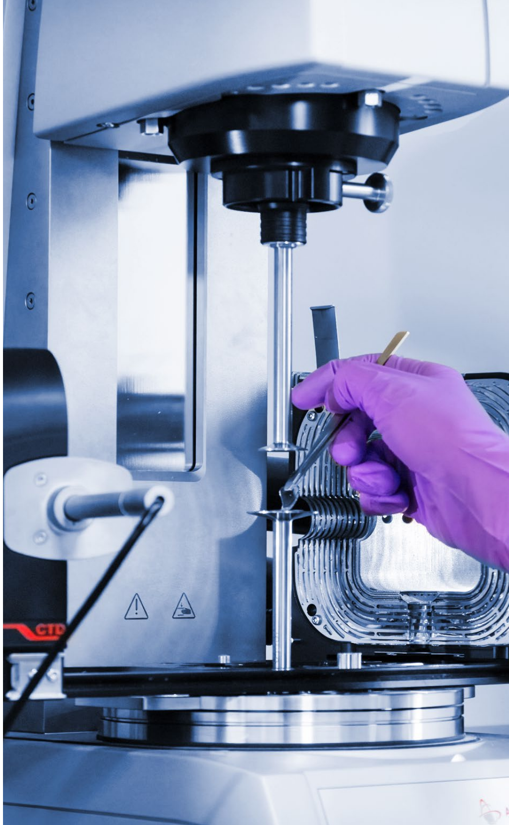
→ The sample is placed within a plate-plate geometry
