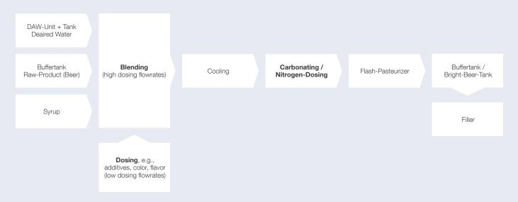
Integrate any Flex-Blend 7000 series' module into any comprehensive system – the blender, carbonator, flavor dosing, buffer tanks, and water dearation systems are synchronized and operated by a single human machine interface (HMI). Set up the Flex-Blend 7000 series to interact with a supervisory control system for remote operation, or let it control adjoining process systems.
