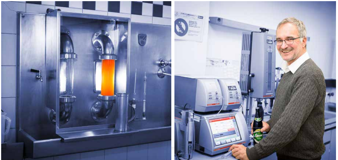
All-rounder: The PBA-B modular measuring system measures up to eight parameters from one beer sample.
