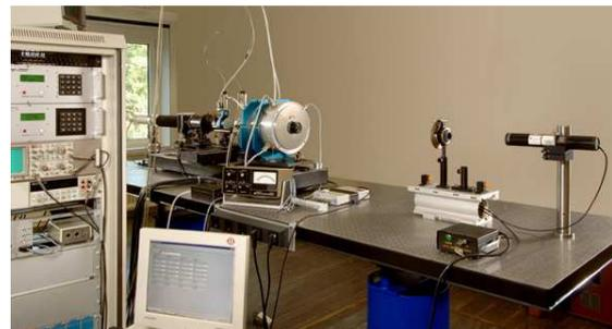
Fig. 1 High precision polarimeter at the PTB. Source: [9]
