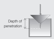
Allow the cone to penetrate the grease for five seconds, then read the depth of penetration.
