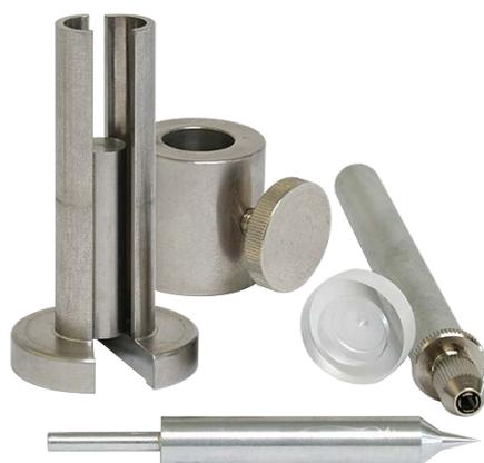
Figure 2 Micro-Cone Test Set
