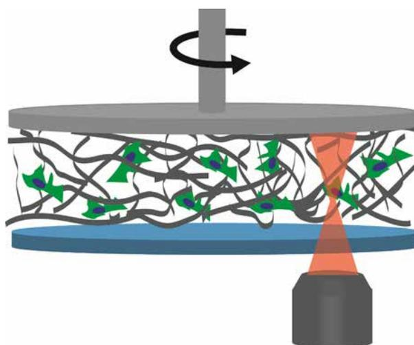
*Figure 1. Schematics of a confocal-rheology experiment, in which a soft polymer (in this case containing cells) is visualized by fluorescence microscope while simultaneously applying strain to the sample by the rheometer plate on top.*
