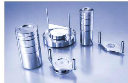
Bench and weights for the small and large shear cell for time consolidation without blocking your device
