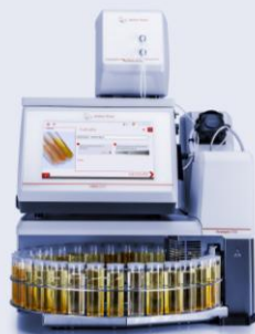
Turbidity measurement system
