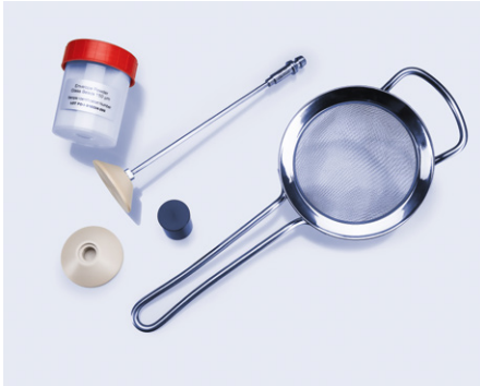
A simple and safe measurement method for characterizing the envelope density of solids with a sample size ranging from 0.3 cm³ to 25 cm³ using a reusable, free-flowing displacement powder. Precise volume measurement with a repeatability of up to 1 % is ensured with a sample quantity of at least 25 % of the total filling volume. In combination with gas pycnometry measurements, the absolute density, porosity, and specific pore volume of solid materials can be determined.
