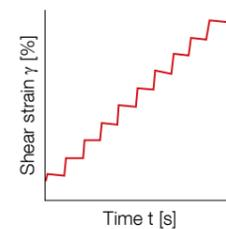
**Multiple stress creep recovery (MSCR) according to AASHTO T350 / ASTM D7405 / DIN EN 16659**
