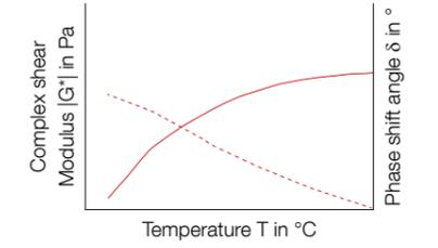
**Determination of temperature-dependent rheological behavior of asphalt binders according to DIN EN 14770**
