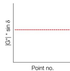
**Superpave performance grading according to AASHTO T315 / ASTM D7175**
