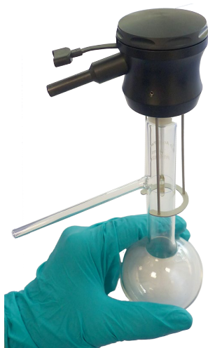
Fig. 7 Multi-plug with protective cage inserted into the flask
