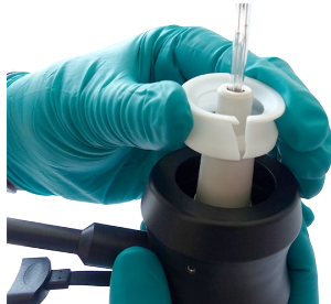
Fig. 3 Extraction of the snap ring
